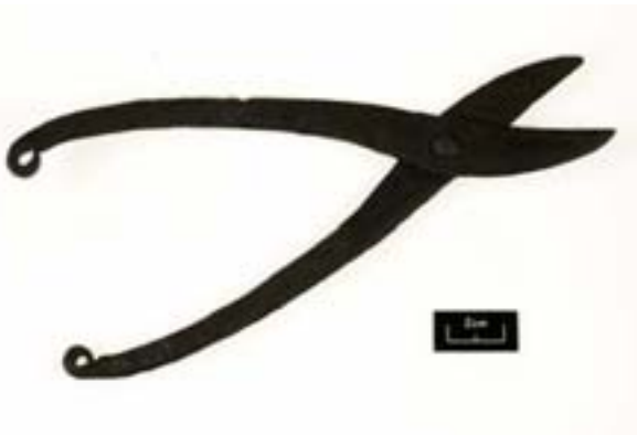
Clippers used for cutting thin sheet metal
